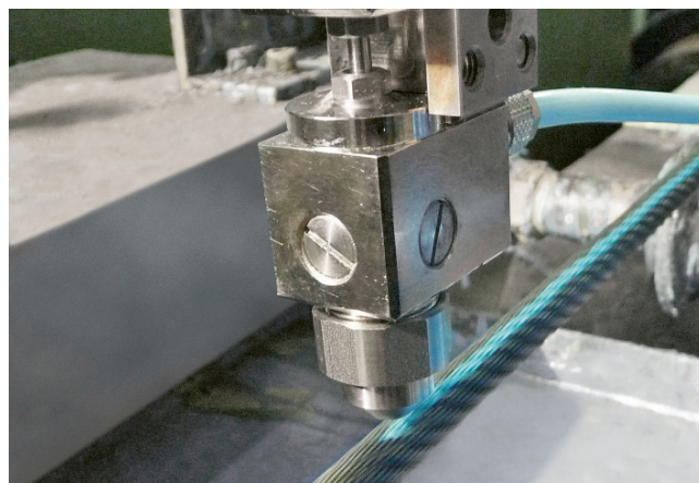
Line marking on steel cables as an assembly aid (swirl marks) for passenger lifts
